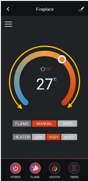
Manually changing the temperature
