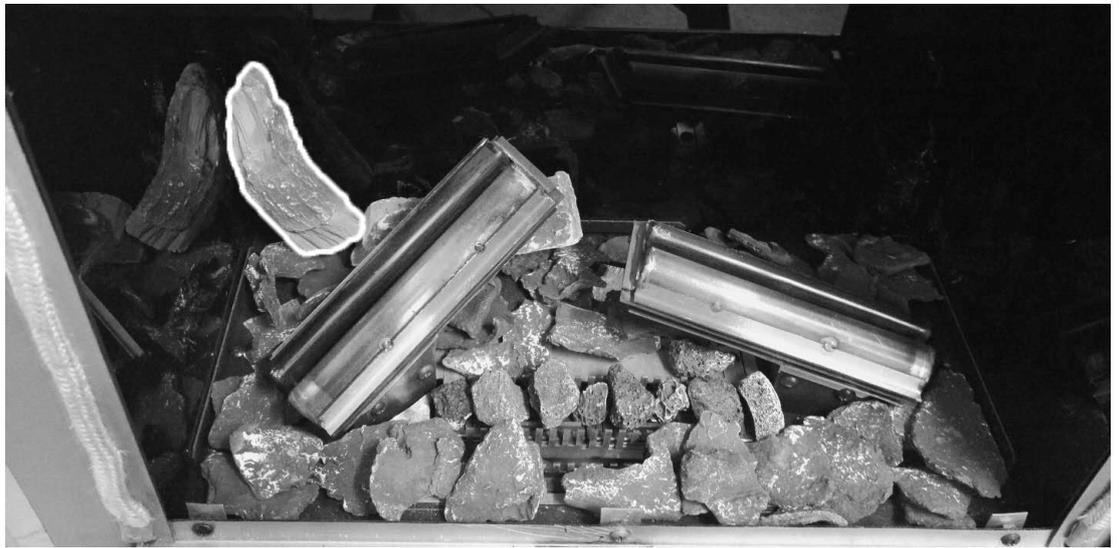
Identify and remove Log E from the ceramic packing carton. Note its orientation for installation in this picture.
