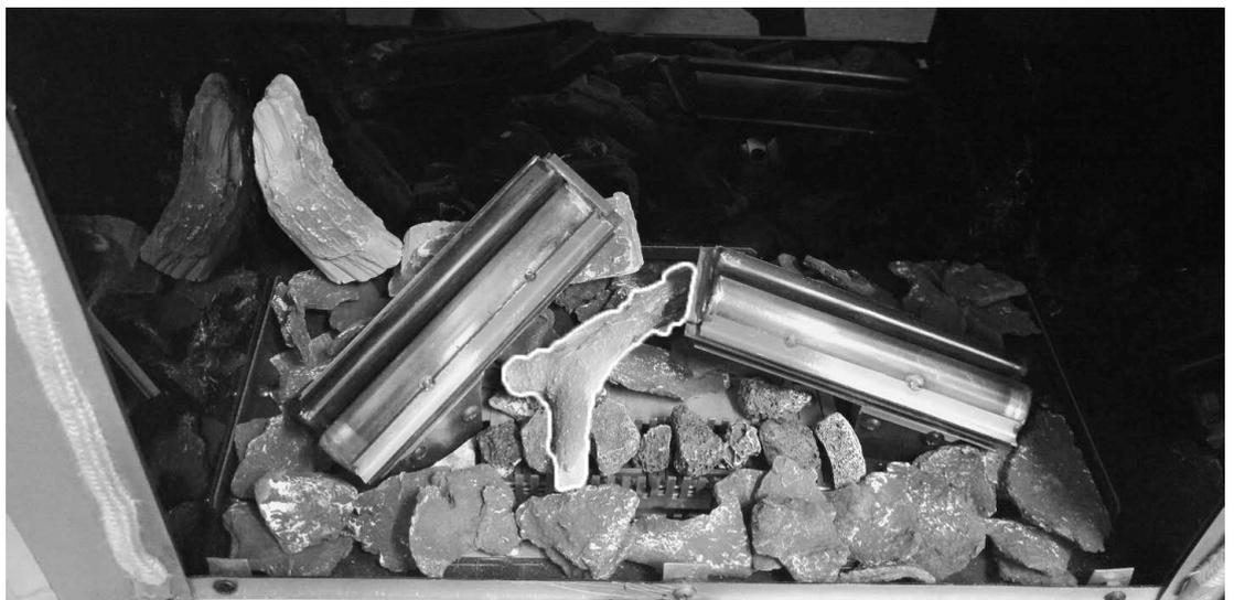
Identify and remove Log A from the ceramic packing carton. Note its orientation for installation in this picture.
