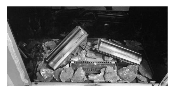
Place the volcanic rock on top of the centre burner as shown. Ensure a 1-2 mm gap is left between each piece. Then using **quarter** of the glowing ember wire supplied, ruffle between fingers to make it loose, about 20mm wide and as long enough to cover the volcanic rock then align over the rock as shown. Ensure no wire is placed within 25mm of the pilot assembly. Retain the rest of the wire for replacement at annual service.
