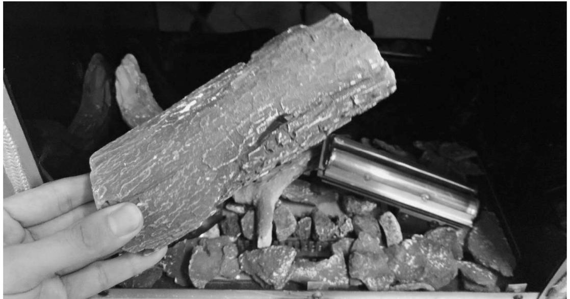
Place log A on the burner tray base at the back of the fire as shown in this picture.
