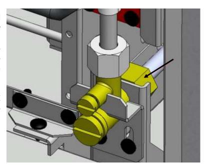
Now carefully lift the appliance into the outer box and guide the horizontal flue section through the outer wall, ensuring the gas supply is sitting in the correct position. The appliance should locate on the two threaded studs at the top left and right of the outer box. Take care that the appliance is fully rearward and these two studs can be seen protruding through their mounting holes.
