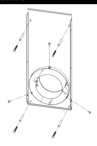
The flue terminal can now be fitted to the outside wall. Ensuring the inner corrugated flue inside the terminal is inserted into the inner horizontal flue, carefully present the flue terminal to the cover plate. Fix the flue terminal to the cover plate using the 6 screws provided—see diagrams below.
