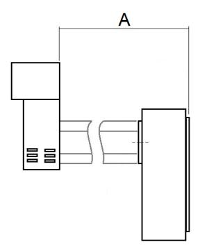
When cutting the horizontal flue section, the outer section can be cut from either side, however whichever side is reduced, the 3 securing holes should be re-drilled, using the off cut section as a guide.
