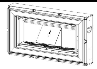
2. Ensure the three panels are pushed together so there is no gap between the panels. Gaps between the panels are not covered under warranty so ensure that these are fitted correctly before proceeding.
