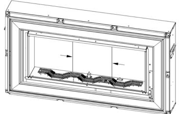
3. Finally, fit the two side glass panels and side liners as shown here. Slide the liner in first and then slide the glass side panel in until it touches the rear glass panels.
