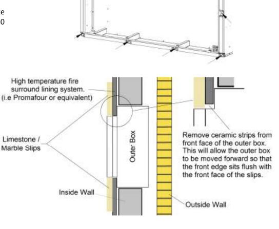
Remove the outer box and drill the hole for the flue (6" diameter) and drill the securing holes with an appropriate masonry drill.
