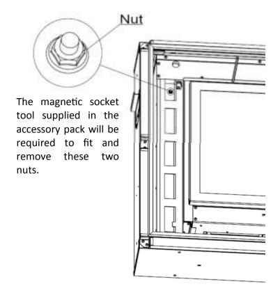
The appliance can now be removed from the outer box. Put the fire aside where it cannot be damaged whilst the outer box is installed into the wall.
