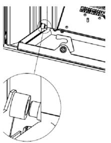
With the door held firmly, slide the glass assembly to the right and it will release from the right hand hinge. Move this corner towards you and the door is now released from the appliance.
