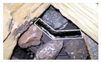
Ensure the secondary airways are not blocked by the volcanic rock
