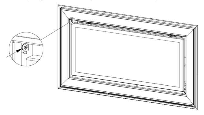
Check that the outer trim assembly is sitting correctly in the slotted brackets located around the entire perimeter of the main trim body.
