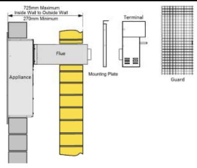
Figure 2 shows the maximum length flue attached to the appliance. If the distance from the front face of the inside wall to the outside wall exceeds 725mm the installation cannot proceed. In most installations the flue section will need to be cut to the appropriate size. Any reduction to flue length must be removed from the end opposite the terminal and the three holes then re-drilled to fix the flue to the appliance—use the holes in the waste section of flue as a guide.
