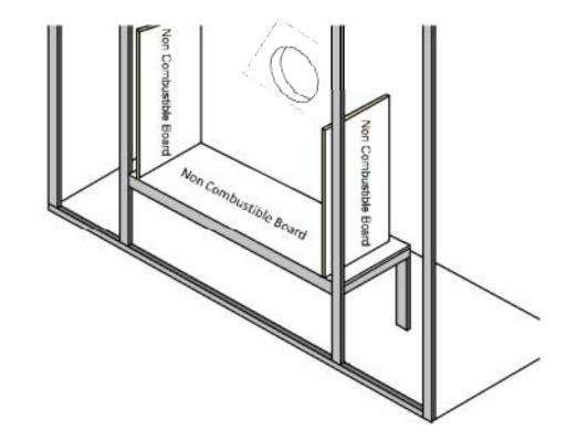
Continue with the installation whilst referring to the cavity wall installation in the previous pages. Again, care should be taken to use a suitable non-combustible board, i.e. Promafour or similar, with no joints around the 'hot area'. This is 500mm above the appliance and 150mm to each side. Fit plasterboard to the front and sides of the chimney breast chamber—ensure an access area is provided for access after installation on one side of this chamber.
