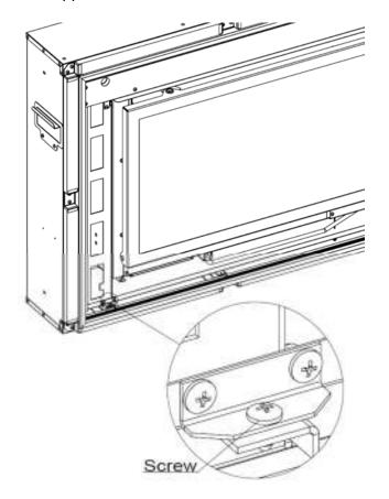
\* These two nuts are not fitted when the appliance is hipped. They can be found in the installation fitting pack.
