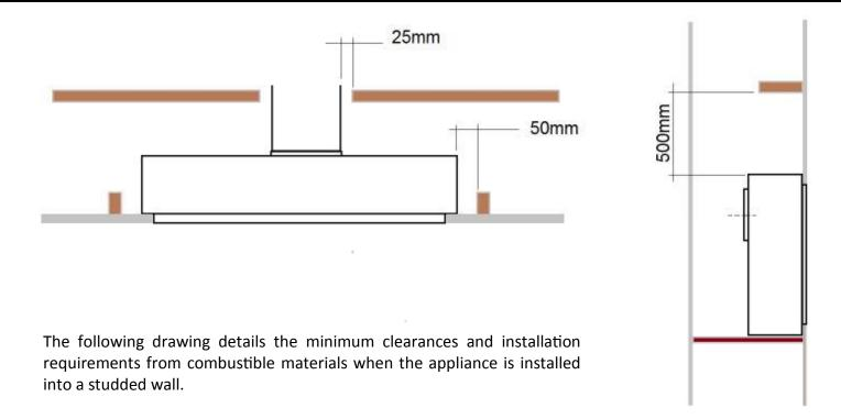
A chamber should be created for the appliance outer box installation. chamber should The be manufactured using non combustible fire-board of minimum thickness of 9mm and the clearances from combustibles (above) should be adhered to. Ensure that the chamber ventilated at the base to allow cool air to enter and ventilated at the top of the chamber to allow warm air to be exhausted into the room. This inlet/outlet vent should have a minimum open area of 100cm<sup>2</sup>.
