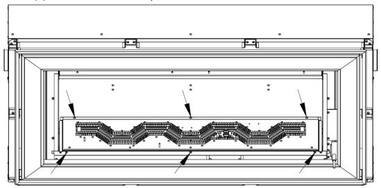
5. Remove the three screws and the burner can be released.
