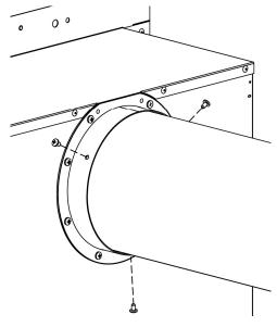
Next, Remove the six screws to release the wall plate from the terminal.
