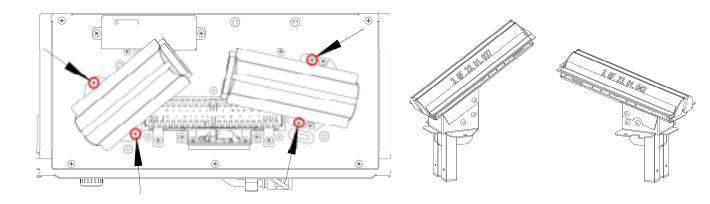
**Now** remove the 4 screws shown to allow the removal of the centre burner
