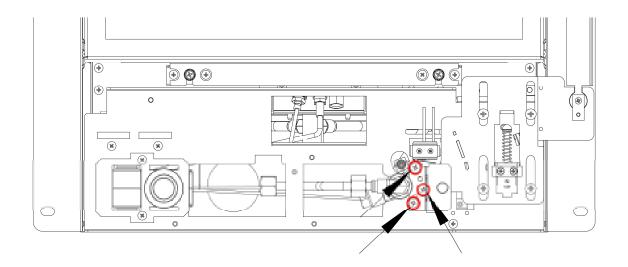
Finally removal of the lock nut at the top of the valve.
