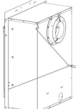
Then pass the other side of wire through the wall eyelet and finally through the lower hole at the front of the appliance.
