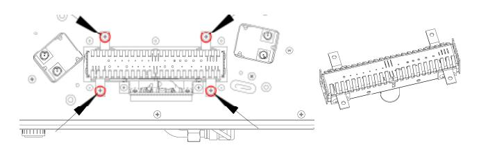
The injectors can be removed or replaced using a 7mm box spanner. Note the location of each injector. Failure to replace the injectors correctly will cause flame and combustion problems.
