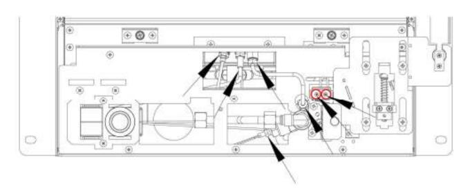
Finally remove the two screws as shown below to remove the Pilot Assembly.
