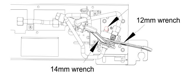
Finally remove the inlet pipe from the tee valve and the valve can then be removed.
