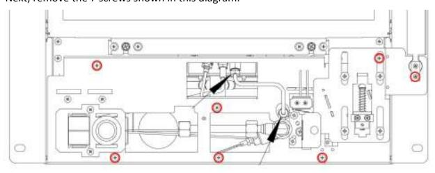
Gently ease the front tray forward, the gas pipes are flexible but take care when moving to ensure the pipes move uniformly as it is removed.
