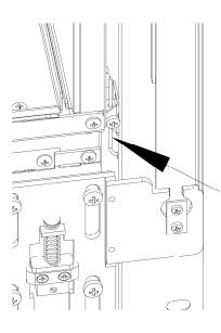
Thread the wire through the hole below the nipple as shown. Pull the wire taut to secure the appliance against the back panel. Finally tighten the small screw on the nipple.
