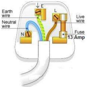
As the colours of the wires in the mains lead of this appliance may not correspond with the coloured markings identifying the terminals in your plug, proceed as follows:
