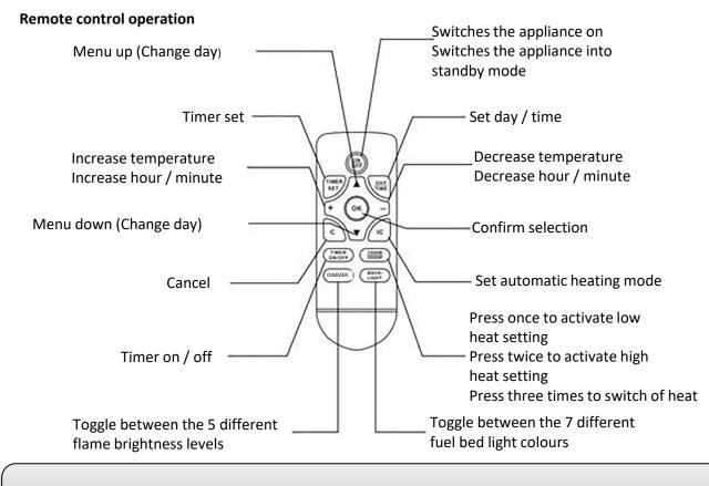
**NOTE:** The heater should be powered on using the Main Power switch before it can be operated using remote control
