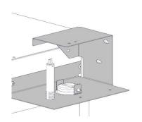
Once in position, mark the position of the 6 x fixing points (3 per side), in the **Support Brackets**.
