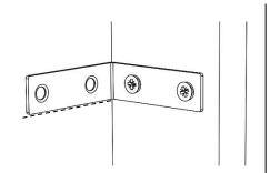
Once in position, mark up the bottom edge of the **Angle Brackets,** pre-installed on the inside of the **Assembled Base**, onto the wall.
