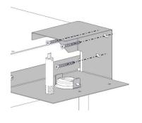
Once the **Fire** and **LED Downlights** are operating correctly, lift the fire back on top of the MDF upstands in the bottom of the **Assembled Base** and offer it into position back up tight against the wall, centralizing the **Fire** on the opening.
