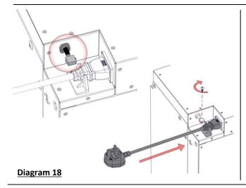
Before proceeding further, position the **Fire** as close to the front of the <u>Assembled Base</u> as possible and ensure the power cable for the **Fire** and the **Fly Lead** for the **Pre- installed LED Light Set** are connected to the **Fire**. (Please refer to **Page 11** in the separate <u>Fire</u> <u>Operating Instructions</u>).
