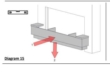
Once the 2 x Wall Brackets are fixed to the wall - lift the Assembled Base back to the wall, ensuring the Angle Bracket and Wall Bracket, engage correctly.
