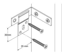
Lift the **Assembled Base** away from the wall and proceed with marking the **2** x **Wall Brackets** fixing positions on the wall. **(Brackets bagged with the surround).**
