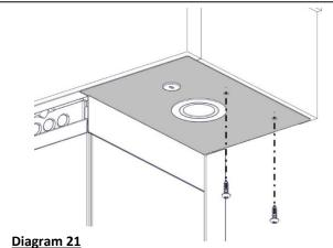
Once centralized, create a pilot hole though the fixing points on the 2 X Support Brackets, into the underside of the Assembled Top. (2 x Pilot Holes per side.)
